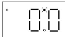
Use the ▲ and ▼ buttons to scroll to the password value (the factory default password is “225”) and press the **Mode** button. Once the correct password value is entered, the display will read “P01”, which indicates that the PROGRAM mode has been accessed at the beginning of the parameter menu (P01 is the first parameter). This is shown below:
