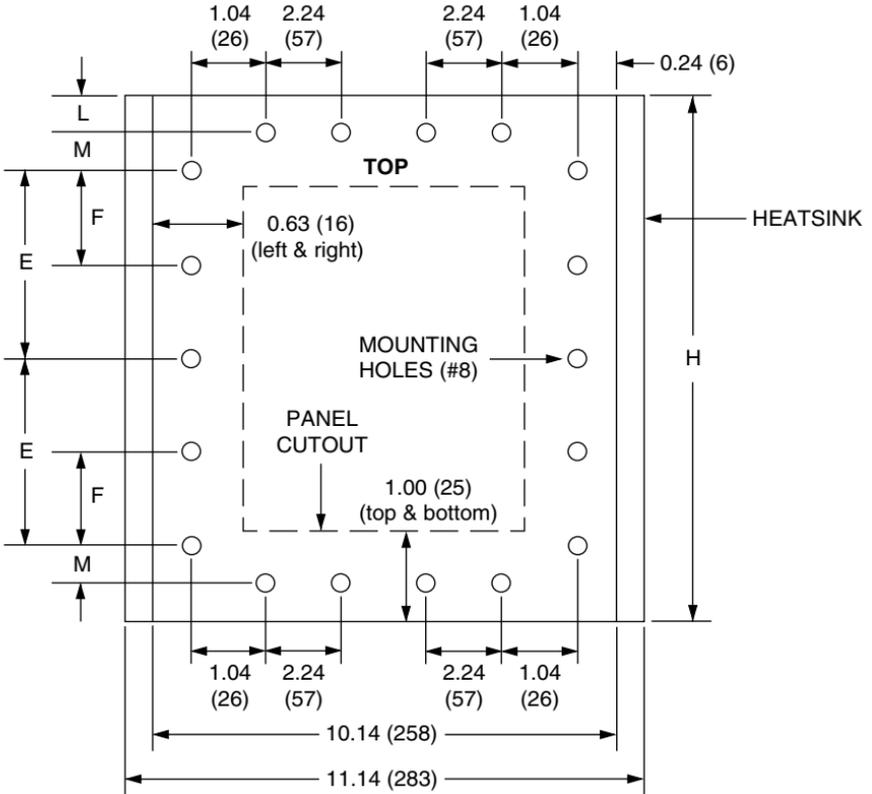
**THROUGH-HOLE CUTOUT DIMENSIONS FOR 15 HP (11 kW) & 20 HP (15 kW) MODELS**
