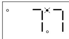
In the example above, Parameter 54 - MOTOR LOAD is being viewed. The “77” in the example indicates that the load on the motor is 77% of the output current rating of the drive.
