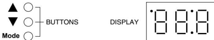
To enter the PROGRAM mode to access the parameters, press the **Mode** button. This will activate the PASSWORD prompt (if the password has not been disabled). The display will read "00" and the upper right-hand decimal point will be blinking, as shown below:
