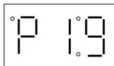
Once the desired parameter number is found, press the **Mode** button to display the present parameter setting. The upper right-hand decimal point will begin blinking, indicating that the present parameter setting is being displayed, and that it can be changed by using the ▲ and ▼ buttons.
