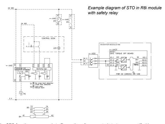
The STO function corresponds to Prevention of unexpected start-up as specified by EN 1037:1995 + A1:2008 and Uncontrolled stop (stop category 0) as specified in EN 60204-1:2006 + AC:2010.
