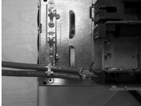
Figure 2-3: Locate Grounding Clamp
