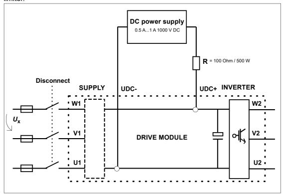
4. Switch on the reforming circuit for the time defined in section *Reforming time* on page 9.
