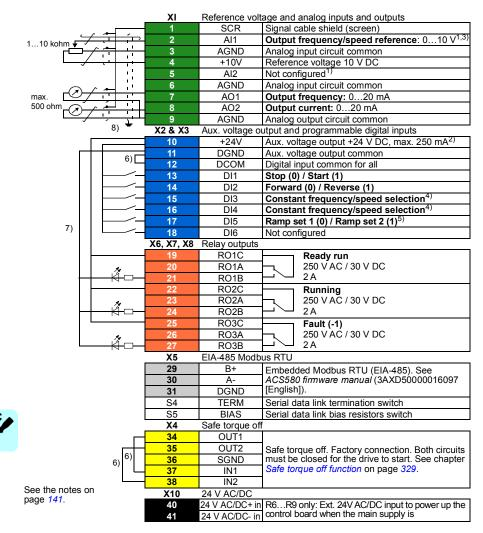
Total load capacity of the Auxiliary voltage output +24V (X2:10) is 6.0 W (250 mA / 24 V DC). Digital inputs DI1...DI5 also support 10 to 24 V AC Wire sizes: 0.14...2.5 mm<sup>2</sup> (26...16 AWG): All terminals Tightening torgues: 0.5...0.6 N·m (0.4 lbf·ft)
