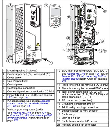
This is an example of IP55 / UL Type 12 frames. They have one-piece front cover, which has a transparent window to leave the control panel visible. UL Type 12 frames have a hood, whose construction depends on the frame size.
