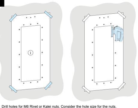
Note: Mounting templates are different (size, number and position of holes) for different frame size.
