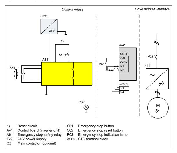
Initial status: The drive is in operation and the motor is running.
