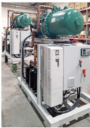
To achieve very accurate control of compressors and pumps, and consequently accurate adjustment of the cooling capacity, Frigel has adopted ABB's ACS580 drive, combined with ACS310 auxiliary units mounted on the pumping groups to circulate the coolant fluid between chiller and users. Each drive is controlled by a PLC programmed with proprietary logic.
