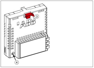
4. Tighten the screw to torque 0.8 N·m using a Torx TX10 screwdriver.
