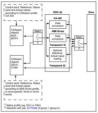
The following sections describe the Control word, the Status word, references and actual values for the CANopen device profile CiA 402 and the ABB Drives communication profile. See the drive manuals for details on the native communication profiles.
