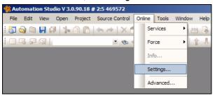
3. Create or modify the connection settings to reflect the serial connection to the PLC. Then, on the Serial tab, right-click the connection and click Connect
