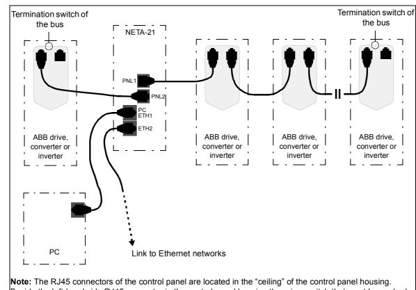
Beside the left-hand side RJ45 connector in the control panel housing there is a switch that must be pushed upwards in the last drive of the chain to terminate the bus.
