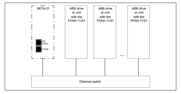
The NETA-21 detects nearby adapter modules (max. 10 pcs over Ethernet) in a local network. The automatic detection is enabled by default only via the ETH2 port. To change the settings of the automatic detection, go to **Settings –> Device interfaces –> Ethernet –> Settings –> Background scan**.
