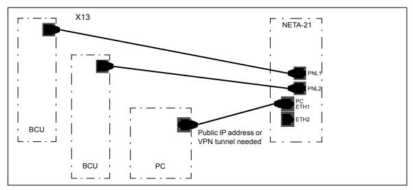
In the BCU-01/02/12/22 control unit, use connector X13 for the panel bus connection.
