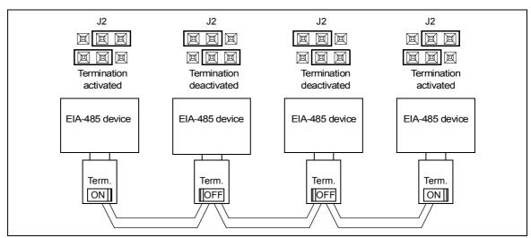
You can use the internal resistor of RS-485/EIA-485 adapters or an external passive termination resistor. The internal termination switch activates also the pull-up and pull-down resistors.
