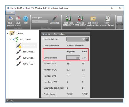
7. The MTQ22-FBP is now configured and should be able to communicate with the PSE.
