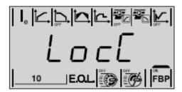
When LocC is selected, the control of the softstarter will automatically switch from fieldbus control to local control. The switch to local control will make hard-wire control possible. When the Fieldbus starts working again the control is automatically switched back to the Fieldbus. There is a 10 second delay before it is possible to controlling the motor.
