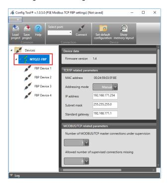
2. From the Select port drop down menu select the COM port associated to the MTQ22-FBP and click connect. The number of the COM port varies, make sure to select the one connected to the MTQ22-FBP.
