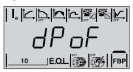
It is possible to read and set this parameter via the keypad when Fieldbus Control is set to On or OFF.
