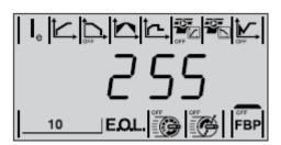
Changing this parameter will automatically reset the fieldbus interface and the new address will be active. If MTQ22-FBP was communicating with the old address, the MTQ22-FBP needs to be re-configured and the PSE restarted.
