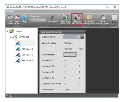
6. Select the FBP Devices in the Config Tool and set the expected Device address to match the Device address read by the MTQ22-FBP. When the two Device addresses match for all connected PSEs click the Write to MTQ22-FBP button again. Note that, when the slave ID is updated in the PSE a reboot will be required on the PSE for the Config Tool to the detect the new value.
