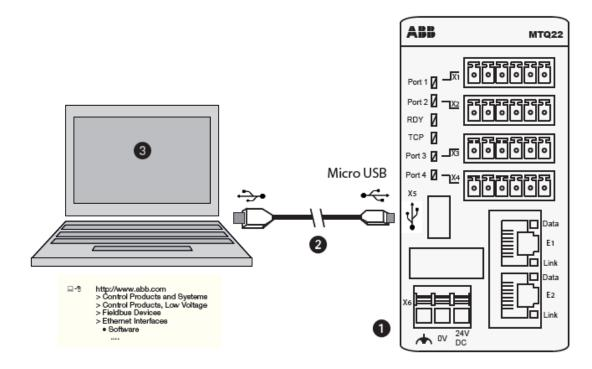
Figure 4: Connecting the MTQ22-FBP to a service Laptop. The MTQ22-FBP must be supplied with 24V DC before the configuration can take place (1). For the connection a Micro USB cable (2) is used. On the PC the MTQ22-FBP configuration software must be installed (3).
