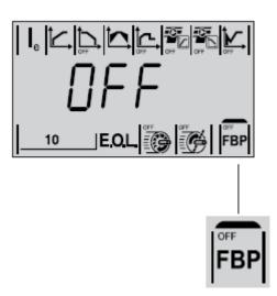
If this parameter is set to On, the softstarter might trip on fieldbus fault if no fieldbus communication is available. If the intention is to run without fieldbus control, this parameter should be set to OFF.
