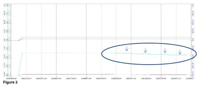
This graph shows the output of the drive. After 50 seconds, Active Energy Control begins to reduce the voltage while continuing to monitor the motor output frequency. The energy savings can be seen on the light blue line (Motor Voltage) as it steps down.
