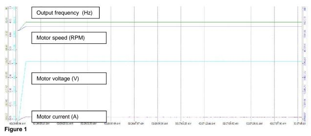
Once the Motor ramps up to 50% speed the output remains constant
