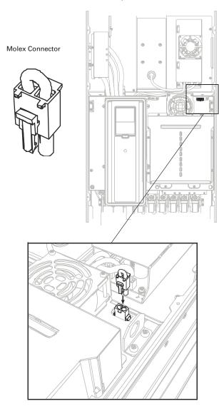
Further remove the extension box cover, the touch shield and the I/O plate with I/O grommet plate. Locate the EMC jumper on the EMC board (see magnification in figure below) and remove it.
