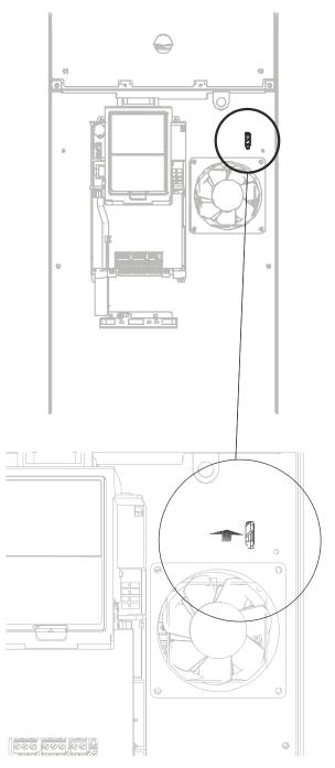
**FS7 and FS8:** Locate the EMC box under the cover. Remove the screws of the box cover to expose the EMC-jumper. Detach the jumper and re-fix the box cover. See figure below.
