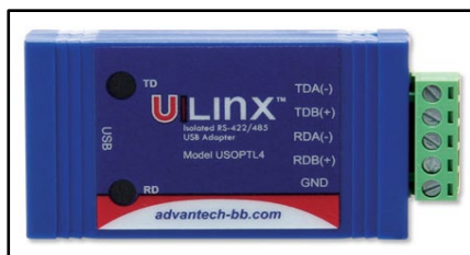
Figure 11: B&B SmartWorx, Inc Model: USPTL4 model RS-422/485 converter
