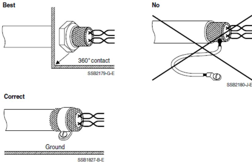
Ensure that an EMC-compliant cable gland is provided at the motor terminal box. It must correspond to the degree of protection for its respective location of use. The motor terminal box shall be made of metal, the connection between cable gland and terminal box must be of large-area design. If the lacquer has been removed, it may be necessary to restore the corrosion-protection layer.
