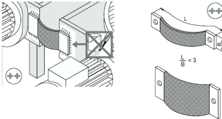
4. Keep cables from the interference source as short as possible!
