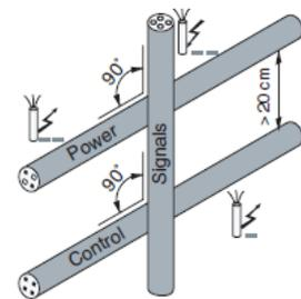
9. In order to reduce interference coupling, as far as possible run the cables close to metal parts which are connected to the reference potential (mounting plates, switch cabinet etc.)
