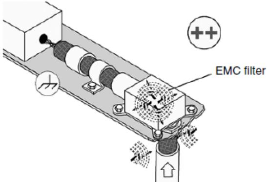
8. Spatial separation between interference-emitting and “clean” cables must be ensured (noisy cables include those between converter and filter, whereas “clean” cables include those between mains supply and filter).
