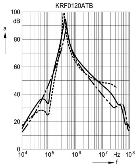
**Insertion Loss (typical values at Z = 50 Ω)**
