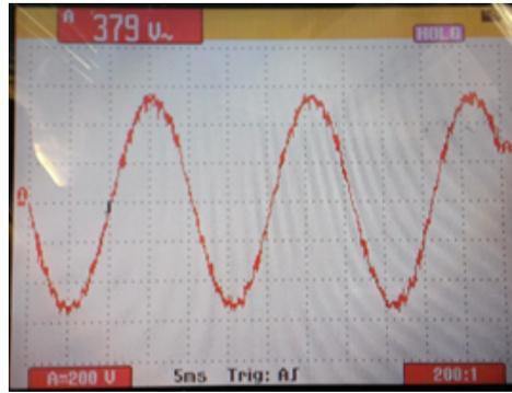
Figure 6: With Sine Filter
