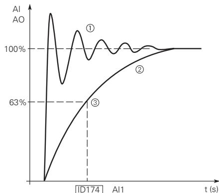
**Notes:** ① Analog signal with faults (unfiltered).
