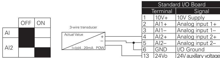
**Figure 54. AI2 4wire-current**
