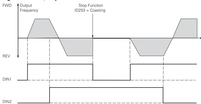
2 = P3.2: DI closed contact = start / open contact = stop P3.3: DI closed contact = start enabled / open contact = start disabled and drive stopped if running Motor direction keeps forward - This would be considered 3 wire control with Start signal 2 required to be closed to enable Start on Start signal 1.
