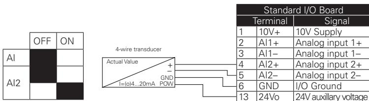
1 = 0-10V - If using the 10V supply on Terminal 1 of the drive, it will require a ground jumper from Terminal 6 to the AI- input terminal 3.
