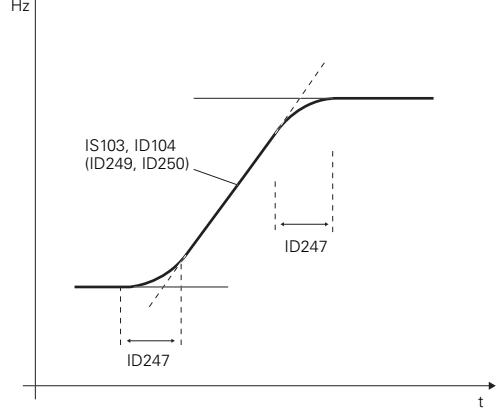
**Figure 79. Acceleration/Deceleration (S-shaped)**
