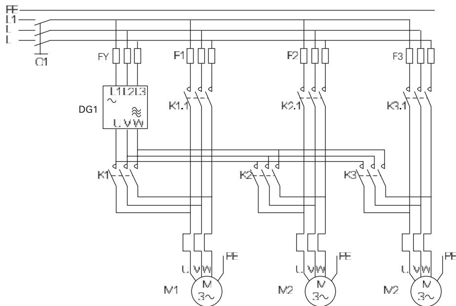
**Figure 30. Three-Pump autochange system principal control diagram**
