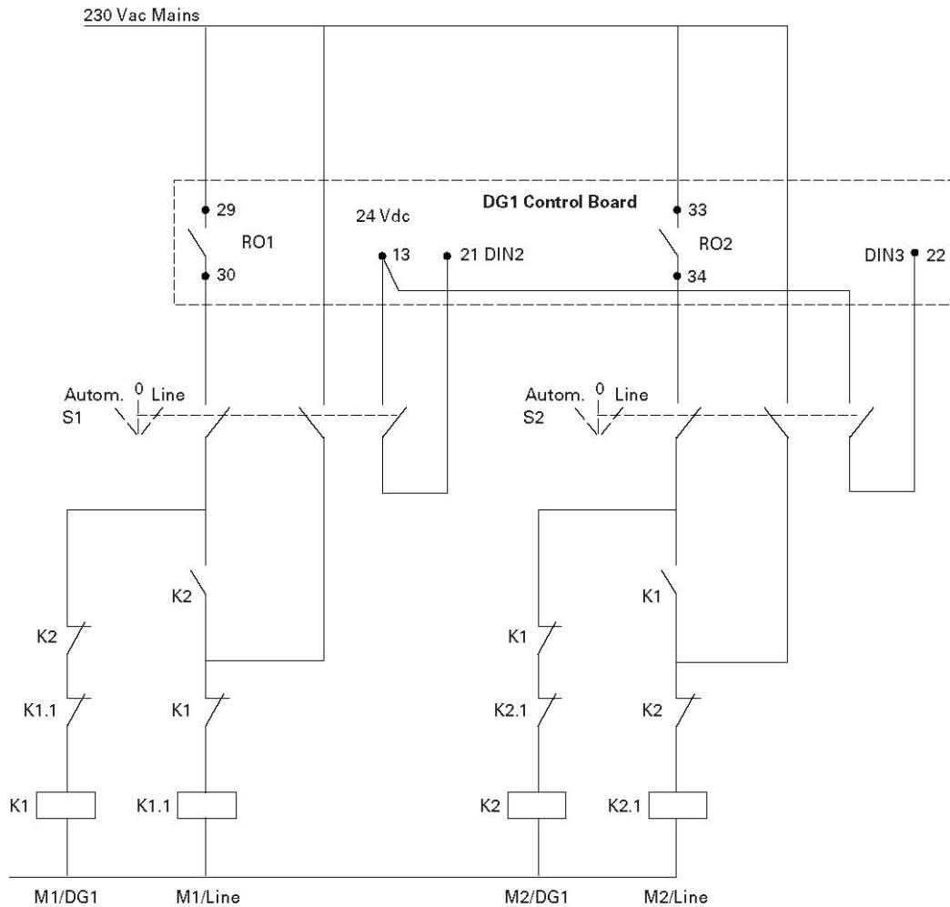
**Figure 29. Example of Three-Pump autochange, main diagram**
