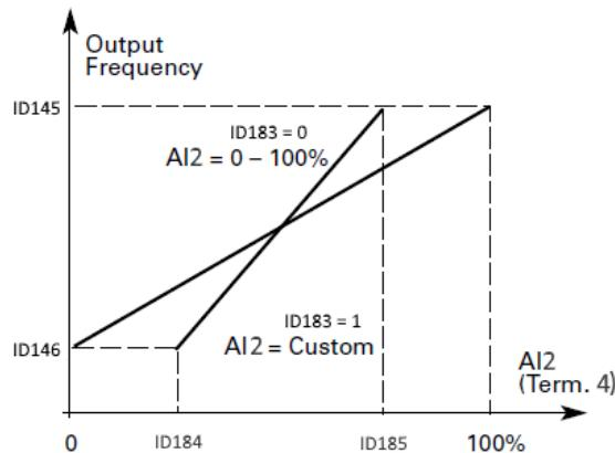
**Figure 59. AI2 Signal inversion**
