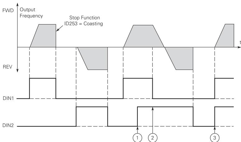
1 = P3.46: DI closed contact = start /open contact = stop P3.47: DI closed contact = reverse / open contact = forward - This would be considered 2 wire control with a contact on start/stop, contact open it stops and direction on 2nd start signal.
