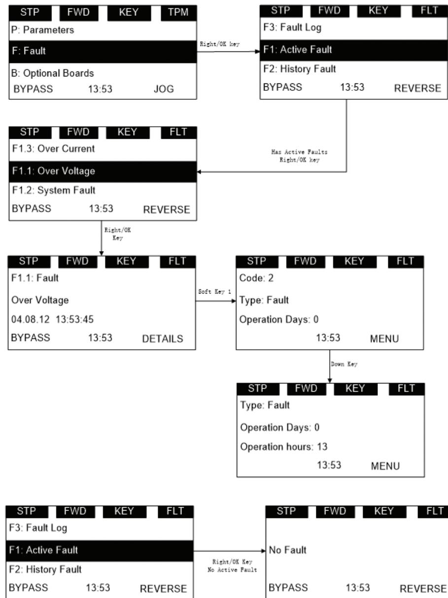
After the DETAIL soft key is pressed, the following detail information about the fault shall be shown: fault code, type, power day count, power hour count, frequency, current, voltage, power, torque, DC voltage, unit temperature, run status, direction, warning, zero speed, Mwh count, at reference.
