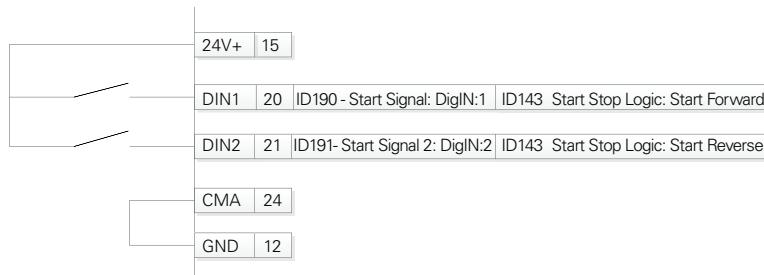
**Figure 62. Start forward/start reverse**
