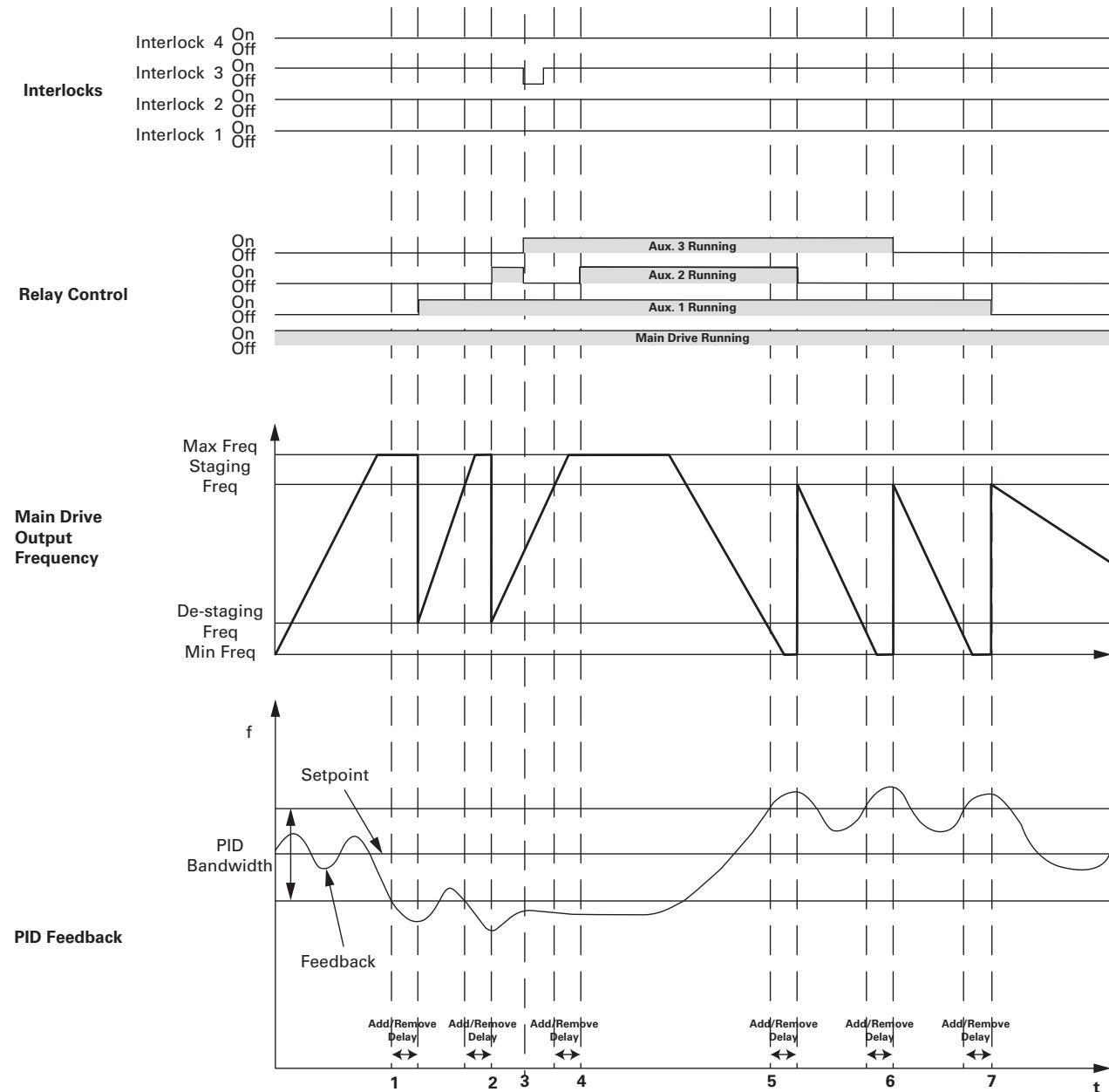
1. Feedback out of bandwidth, output frequency over staging frequency, start delay counter; delay times out, and interlock 2 is ok, add aux 1 motor by closing its corresponding relay.
