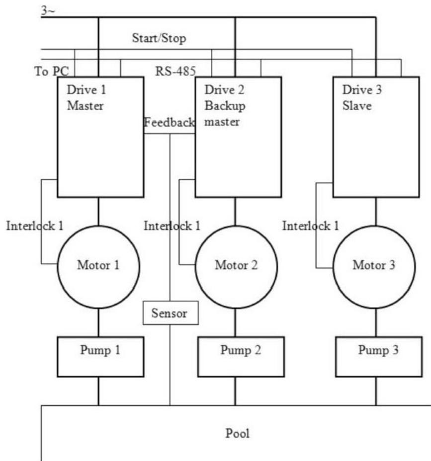
**Figure 34. PowerXL drives with 10 V supply with a 0–10 V transducer**
