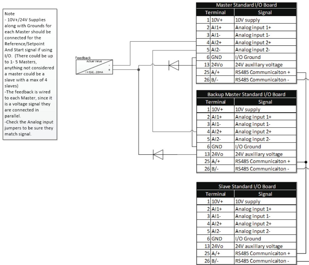
**Figure 36. PowerXL drives with Ext supply with a 4–20 mA transducer**
