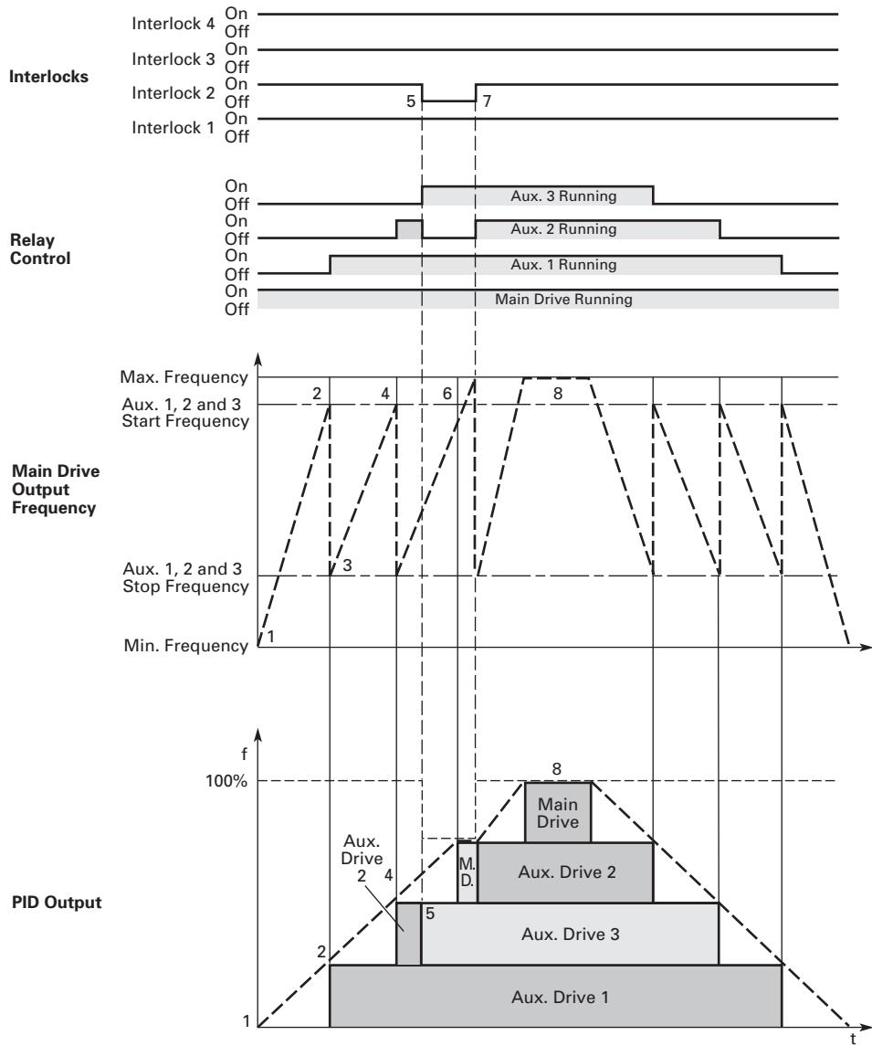
**Figure 32. Multi Pump control curve**
