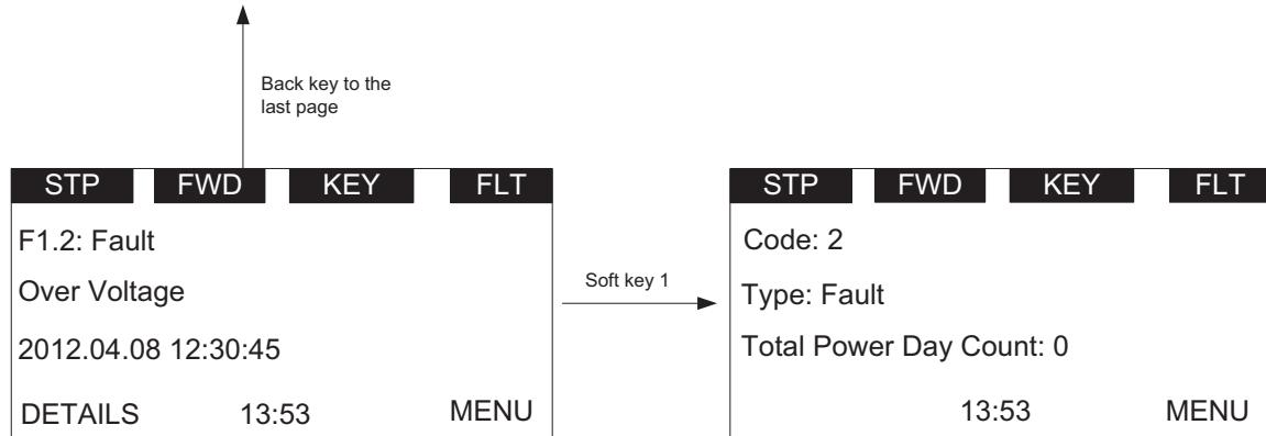
The latest active fault page shall pop up when there is a new active fault, the pop-up fault page is the same as the active fault page.
