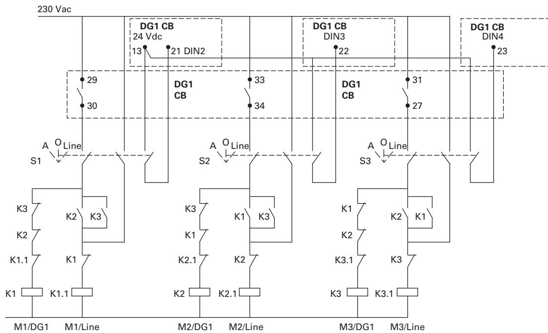
**Figure 31. Example of the function of the PFC application with three auxiliary drives**
