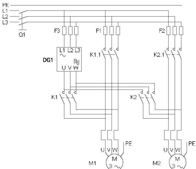
**Figure 28. Two-Pump autochange system principal control diagram**
