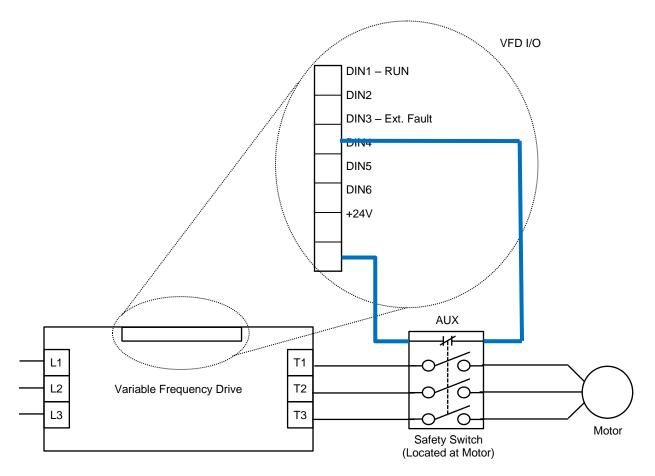
Figure 2 - Interlocking with the VFD EXTERNAL FAULT Input
