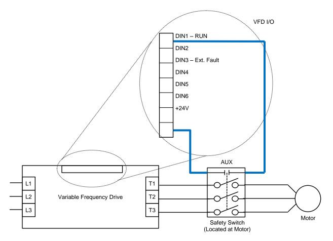
Figure 1 - Interlocking with the VFD RUN input
