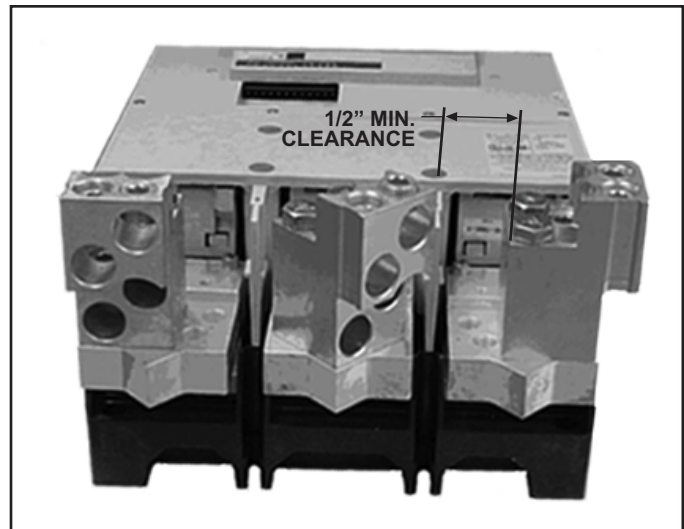
Fig. 2 S801V Shown with EML40 Lugs Installed on Load Side - Terminal Cover Cannot be used with EML40 Kit.
