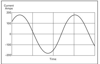
Figure 31.0-15. 100 hp 480 V Drive with 18-Pulse Rectifier
