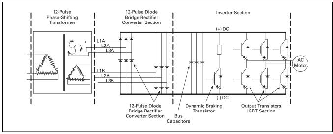
Figure 31.0-14. Basic 12-Pulse Rectifier with "Phase-Shifting" Transformer
