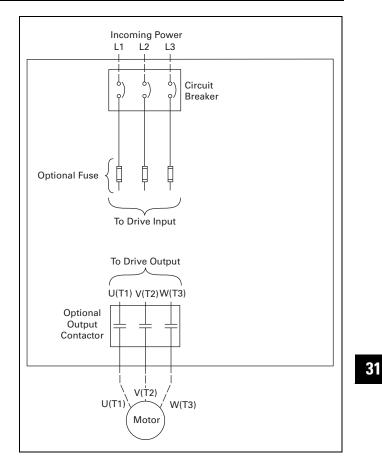
Figure 31.3-5. H-Max Series IntelliDisconnect Power Wiring
