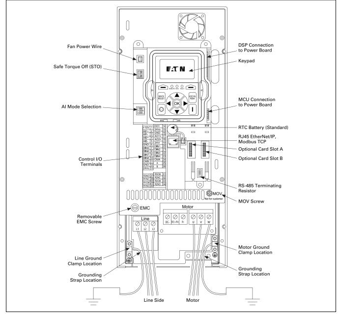
Figure 31.1-5. PowerXL Series—DG1 Control Board Layout
