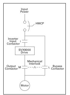
Figure 31.2-19. Power Diagram for Bypass Options RB and RA
