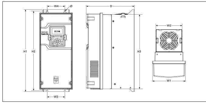
Figure 31.1-6. PowerXL Series—DG1 Dimensions
