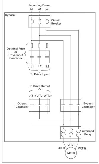
Figure 31.3-4. H-Max Series IntelliPass
