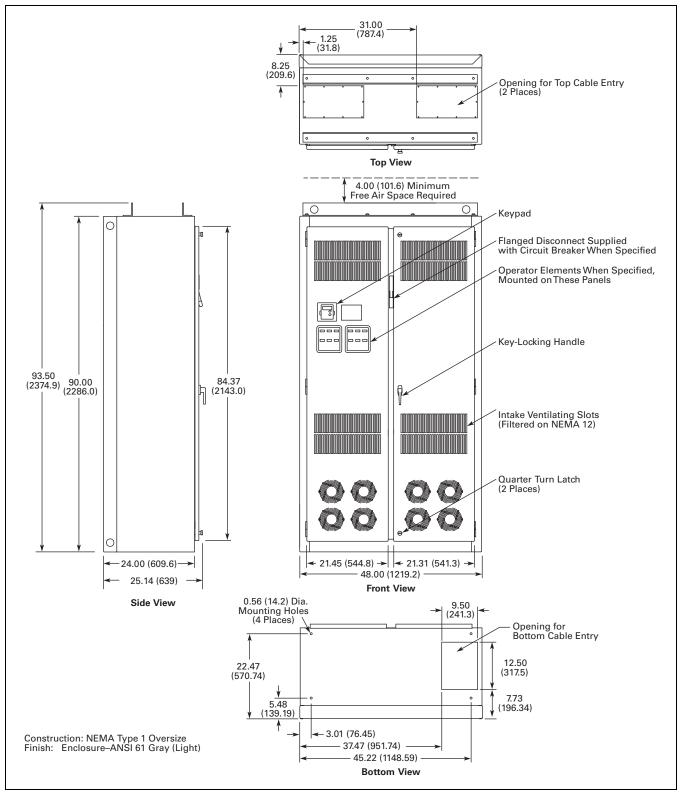
Figure 31.2-44. 200–250 hp I<sub>L</sub> and 150–200 hp I<sub>H</sub>—Approximate Dimensions in Inches (mm)
