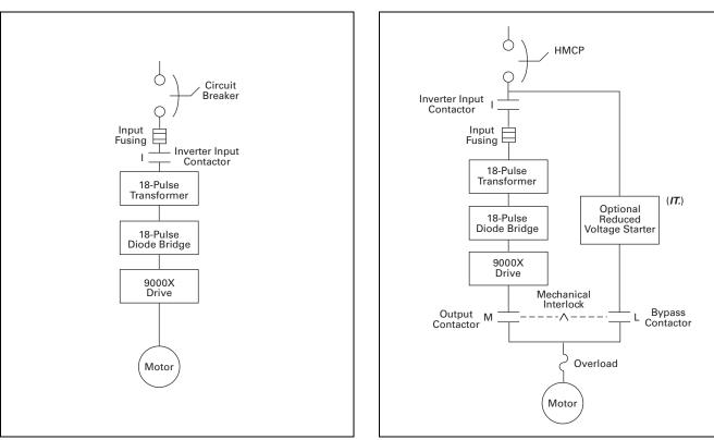
Figure 31.2-47. Power Diagram 25–250 hp IL and 25–200 hp IH
