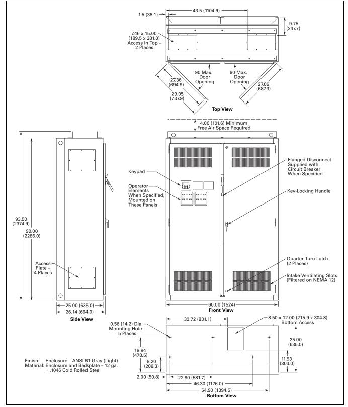
Figure 31.2-45. 300–400 hp IL and 250–350 hp IH—Approximate Dimensions in Inches (mm)
