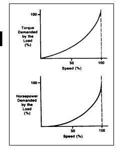
Figure 31.0-3. Variable Torque Load
