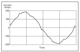
Figure 31.0-11. 100 hp Enclosed 480 V Drive with Integrated Passive Filter
