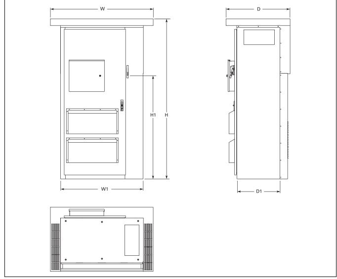
Figure 31.2-32. Enclosure Size F—Approximate Dimensions in Inches (mm)
