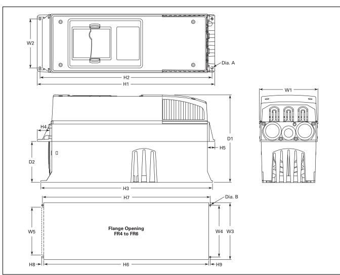
Figure 31.2-3. NEMA Type 1/IP21 and NEMA Type 12/IP54 with Flange Kit, FR4, FR5 and FR6
