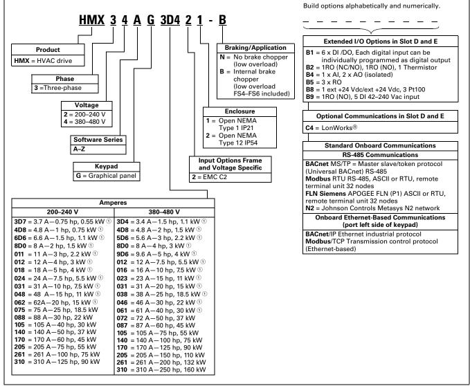
① DB chopper standard frames FS4–FS6. 1.5–40 hp, 3.4–61 A, 480 Vac; 0.75–20 hp, 3.7–62 A, 200–240 Vac.
