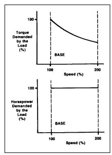
Figure 31.0-2. Constant Horsepower Load
