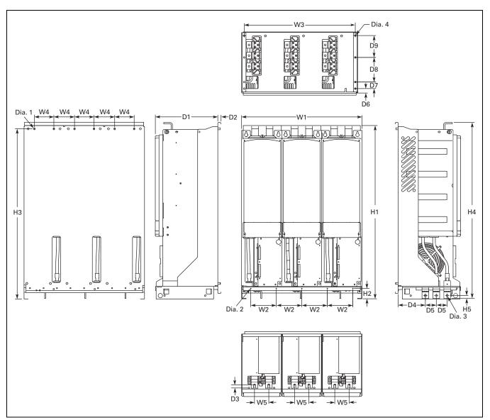
Figure 31.2-15. FR13, Open Chassis Converter—900/1000 hp 480 V
