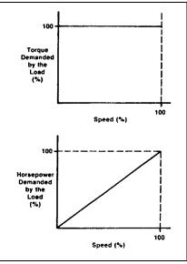
Figure 31.0-1. Constant Torque Load
