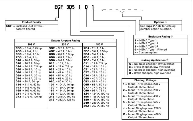
① Brake chopper is a factory-installed option only. Braking resistors sold separately. See DG1 drives starting on Page 31.1-31 for selection.
