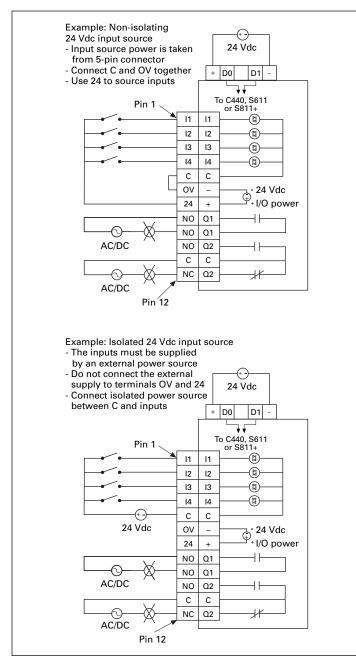
Figure 2. C441QS-24 Vdc input specification
