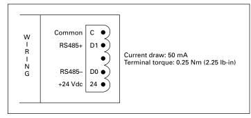
Figure 3. 5-pin 24 Vdc power, RS-485 connector
