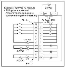
Figure 1. C441SS-120 Vac input specification
