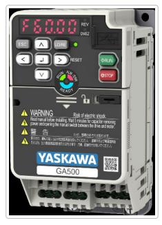
Image: A Yaskawa GA500 series VFD (Variable Frequency Drive). The GA500 is a compact industrial microdrive covering 1/8 to 40 HP, known for its intuitive interface (note the simple keypad and status ring) and flexible networking options. Yaskawa drives like this include built-in safety and are designed for easy setup and high reliability. <sup>26</sup> <sup>24</sup>
