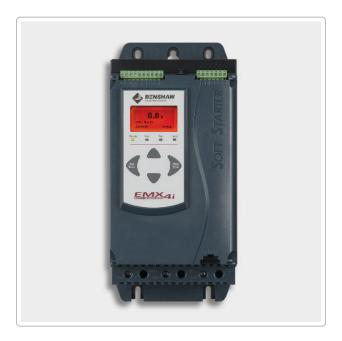
Figure: The Benshaw EMX4i soft starter (front view) features a built-in multi-language graphical display and keypad for configuration and monitoring. These compact devices support motor currents up to 1,200 A ( $\approx$ 900 HP at 460 V) in a single unit. The EMX4i's modular design with pluggable terminals and optional expansion cards simplifies installation and integration into control systems.
