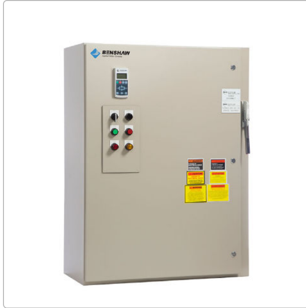
Figure 1: A Benshaw RX4E Series soft starter (75 HP model) in a NEMA-12 enclosure. The door-mounted operator interface includes a keypad (top) for the EMX4i controller, start/stop pushbuttons (green/red), a white local/remote selector switch, indication lights (running and fault), and an external handle on the right for the built-in circuit breaker disconnect. This packaged design simplifies installation and provides safety and control at the panel.
