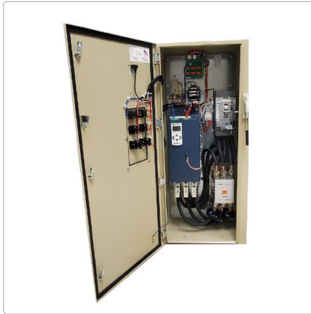
Figure 2: Internal view of a Benshaw RX4E soft starter package (door open). On the right is the integrated circuit breaker (with its handle mechanism visible on the door) and below it the heavy-duty bypass contactor (orange Benshaw label). In the center, the blue module is the EMX4i soft starter controller (connected to the three-phase motor leads via SCR power modules and fuses at its base). The black units on the left door interior are additional control relays and terminals. This layout illustrates the combination starter design – breaker, soft starter, and contactor all contained in one unit – ensuring compactness and coordinated operation.
