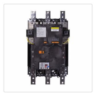
Figure: Eaton S611 soft starter unit (414 A model). The S611 integrates the SCR power devices, a built-in bypass contactor, and an electronic overload relay into one compact unit. This design minimizes the need for external components and wiring, saving panel space and cost while reducing heat dissipation once the motor is at full speed. <sup>3</sup>
