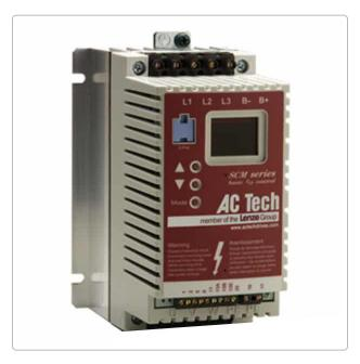
A Lenze-AC Tech SCM series VFD unit. The SCM drives are compact and designed for panel mounting (IP20 enclosure). They feature a basic built-in keypad and 3-digit LED display for programming and monitoring, along with easily accessible terminals for line input (L1, L2/N, L3), DC bus connections (B+, B- for dynamic brake), and motor output. This sub-micro drive exemplifies the flexible, simple, and robust design of the SCM series.
