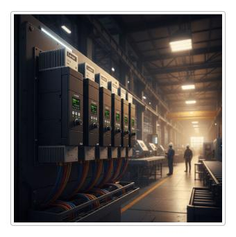
Lenze i550 Protec drives with high IP66/NEMA 4X enclosures can be mounted directly on machinery in harsh factory environments. This decentralized design reduces the need for large control cabinets and long shielded motor cables.
