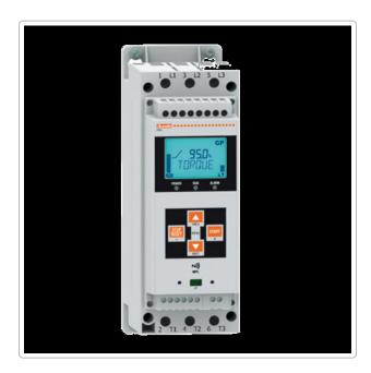
An ADXL series soft starter by Lovato Electric. The compact open-chassis design (IP00) is intended for panel installation. A backlit LCD display and control keypad on the front panel allow easy setup and monitoring, while built-in and optional communication interfaces enable advanced programming and integration.
