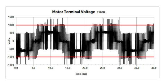
Without a sine wave filter, a VFD's PWM output (shown here at a motor 1500 ft away) contains high-frequency pulses and overshoot voltages that can reach  $\sim$ 3× the nominal voltage, stressing motor insulation 1.
