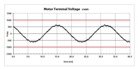
With a TCI KMG Sine Wave Filter in place (same 1500 ft cable), the output voltage is smoothed into a near-ideal sinusoidal wave. The filter removes the carrier frequency, preventing reflective wave spikes and virtually eliminating dV/dt stress on the motor 6.
